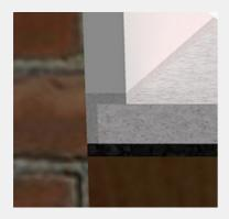
**2.** Add perimeter flanking strip to wall in preparation for SoundScreed being fitted.
